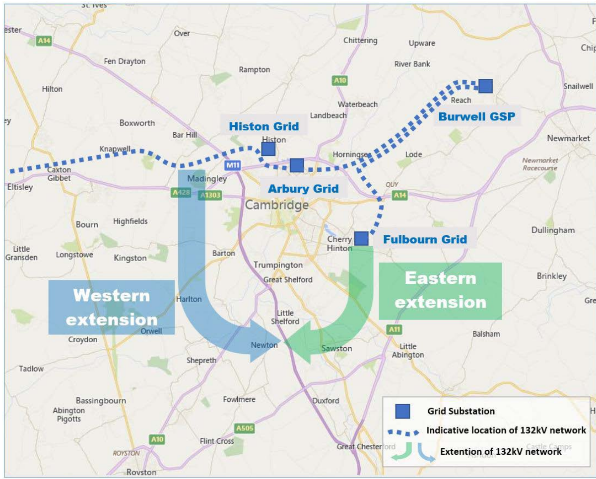
Figure 2 - Existing 132kV network in the Greater Cambridge area and proposed extension corridors
