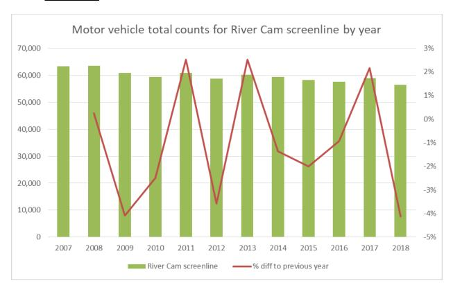
This indicator is from from 12 hour two-directional video surveys conducted between 7am and 7pm once annually on a neutral day in Spring on 5 road bridges over the River Cam with Cambridge.
