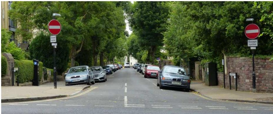
Figure 18 – Example of a One-Way TRO restriction
