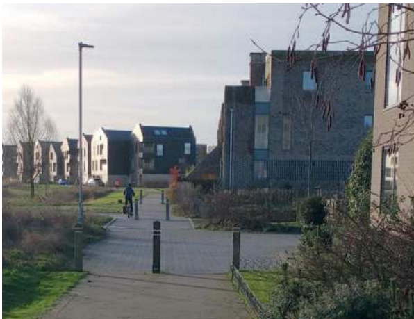
Photo 27a: Modal filtering used (using removable bollards to allow emergency access) along road to prevent through vehicular traffic, Clay Farm, Cambridge.
