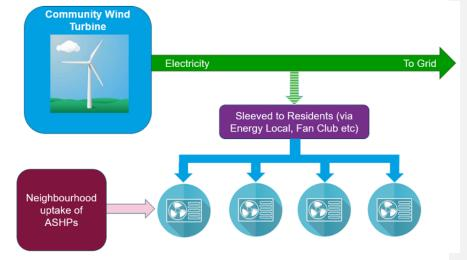
6.6.2 A study on this concept by Possible<sup>14</sup> concluded that a wind turbine could provide 68% of the electricity demand from heat pumps and deliver a 26% cost saving relative to gas heating. The same concept is also possible with solar PV, instead of wind, although Possible found that solar PV generation alone was less well matched than wind with the timing of heat demand. The report found that adding 3 kW rooftop solar PV per
