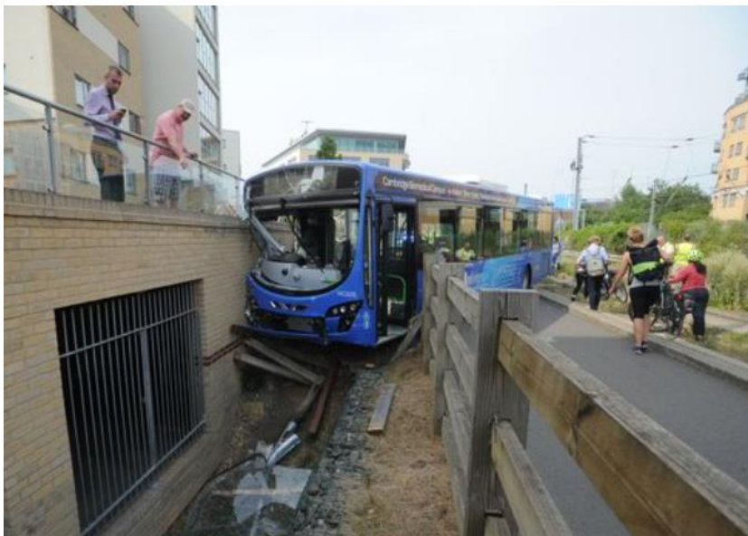
Figure 16.3: Guided Bus Accident as a Result of Avoiding Non-Motorised Users
