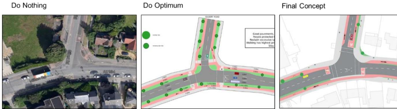
In reviewing the 'Do Optimum' junction layout, it was identified that the suggested radiuses of the junction were too tight to allow for all vehicle turning movements and hence the corner radii need to be relaxed. As a result this would impact on the space available for cycle and pedestrian movements.
