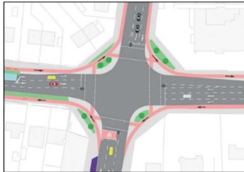
The layout of the 'Do Optimum' signalisation design fails to adequately accommodate all turning movements and needs a larger carriageway area which, in turn, reduces the space available for cycling and pedestrian movements, as indicated within the proposed 'Final Concept' junction design. However, officers believe that many of the ideas for segregating cycle movements from motorised traffic are worth further consideration as the detailed design is developed.
