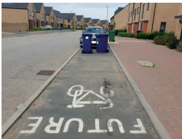
Photo 43: Due to poor planning, cycle lanes are being obstructed by parked cars and bins, Northstowe Phase 1.
