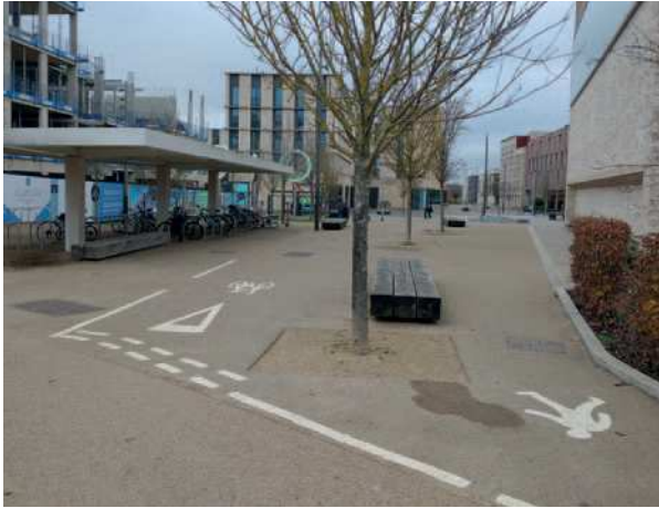
Photos 23a & 23b: Junction of off-road shared paths where segregation and give way lines have been introduced retrospectively to reduce conflict between users in Eddington, Cambridge.
