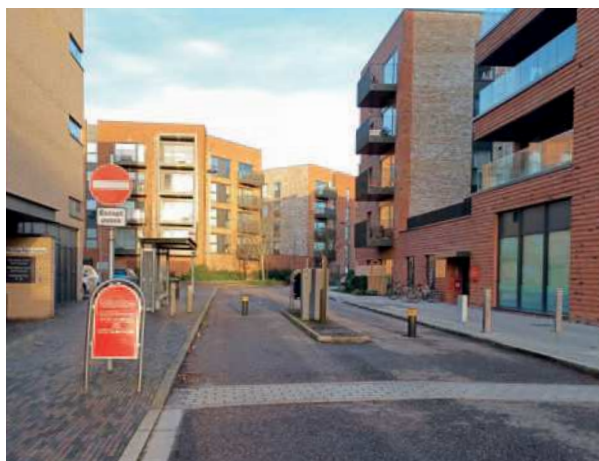
Photo 24b: Permanent restriction on primary road through the Clay Farm development to prevent through traffic.
