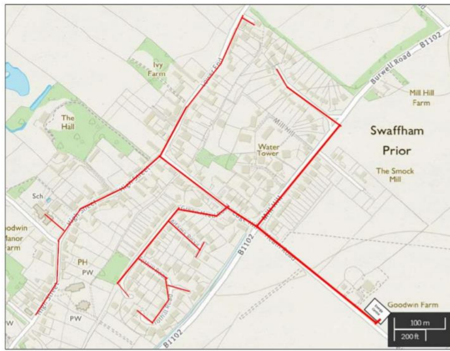
Figure 1: A map of the heat network at Swaffham Prior, with hot water pipes (red) extending from the energy centre (white) underneath the roads to all the houses in the village
